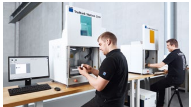
You can also use the TruMark Station 3000 as a desktop workspace or as a stand-alone solution – the supply unit and extractor are integrated into the substructure.
